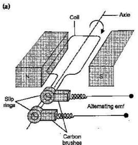
It works on the process of electromagnetic induction, *i.e.*, when a coil rotates continuously in a magnetic field, the effective area of the coil, linked (normally) with the magnetic field lines, changes continuously with time. This variation of magnetic flux with time results in the production of a (alternating) emf in the coil.
