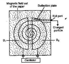
The Ds are the semi-circular structures (D<sub>1</sub> and D<sub>2</sub>) between which the charges move. The accelerating voltage is maintained across the opposite halves of the Ds.
