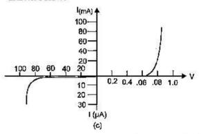
From the V-I characteristics of a junction diode, it is clear that it allows the current to pass only when it is forward biased. So when an alternating voltage is applied across the diode, current flows only during that part of the cycle when it is forward biased.
