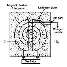
Square wave electric fields are used to accelerate the charged particles in a cyclotron.
