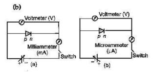
Using the circuit arrangements shown in fig (a) and fig (b), we study the variation of current with applied voltage to obtain the V-I characteristics shown below.
