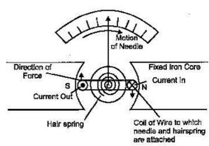
**Principle:** The working is based upon the principle, when a current carrying coil suspended in a magnetic field experiences a torque.
