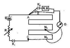
When  $K_2$  is open, balance length is obtained at length  $AN_1 = l_1$
