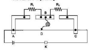
Answer: (a) Working principle of Potentiometer: When a constant current is passed through a wire of uniform area of cross-section, the potential drop across any portion of the wire is directly proportional to the length of that portion.
