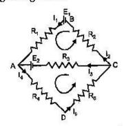
For closed part BACB,  $E_1 - E_2 = I_1R_1 + I_1R_2 - I_3R_3$ For closed part CADC,  $E_2 = I_3R_3 + I_4R_4 + I_5R_5$
