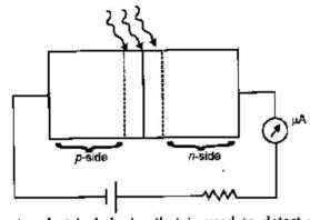
An electrical device that is used to detect and convert light into an energy signal with the use of a photo detector is known as a photodiode. The light that falls on it controls the function of pn-junction. Suppose, the wavelength is such that the energy of a photon  $\frac{hc}{\lambda}$  is enough to break
