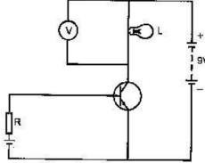
Answer: The given figure is Common Emitter (CE) configuration of an *n-p-n* transistor. The input circuit is forward biased and collector circuit is reverse biased.
