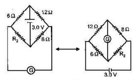
For the equivalent circuit, when the Wheatstone bridge is balanced, there will be no deflection in the galvanometer.
