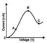
Answer: Resistance of a material can be found out by the slope of the V-I curve. Part BC of the curve shows the negative resistance as with the increase in voltage, current decreases.
